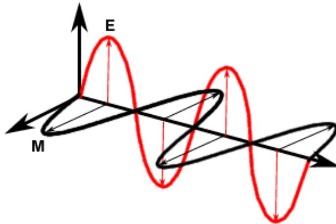
In co-polarization, both Transmit and Receive are sent in the same physical plane (both horizontal or both vertical).
