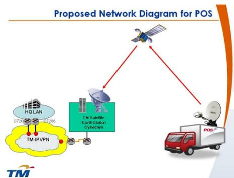
The mobile unit with C-COM's **iNetVu**<sup>®</sup> antenna system installed can be moved to any location in Malaysia. Once the vehicle reaches the site, a simple press of a button gets the antenna automatically pointed to the desired satellite. Traffic from the mobile unit goes up to the satellite and from there down to the Satellite HUB. From the HUB via a backhaul the traffic gets routed to their HQ.
