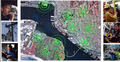
The above figure shows a terrestrial network's coverage in an urban area. The gaps without coverage are easily visible. In rural areas, where many of the mobile post offices would be deployed, the anywhere, anytime connectivity that satellite provides is in most cases the only alternative available. In the case of emergency, such as an earthquake, the only choice of communications is satellite, as it does not depend on the terrestrial infrastructure, which most likely has been destroyed.
