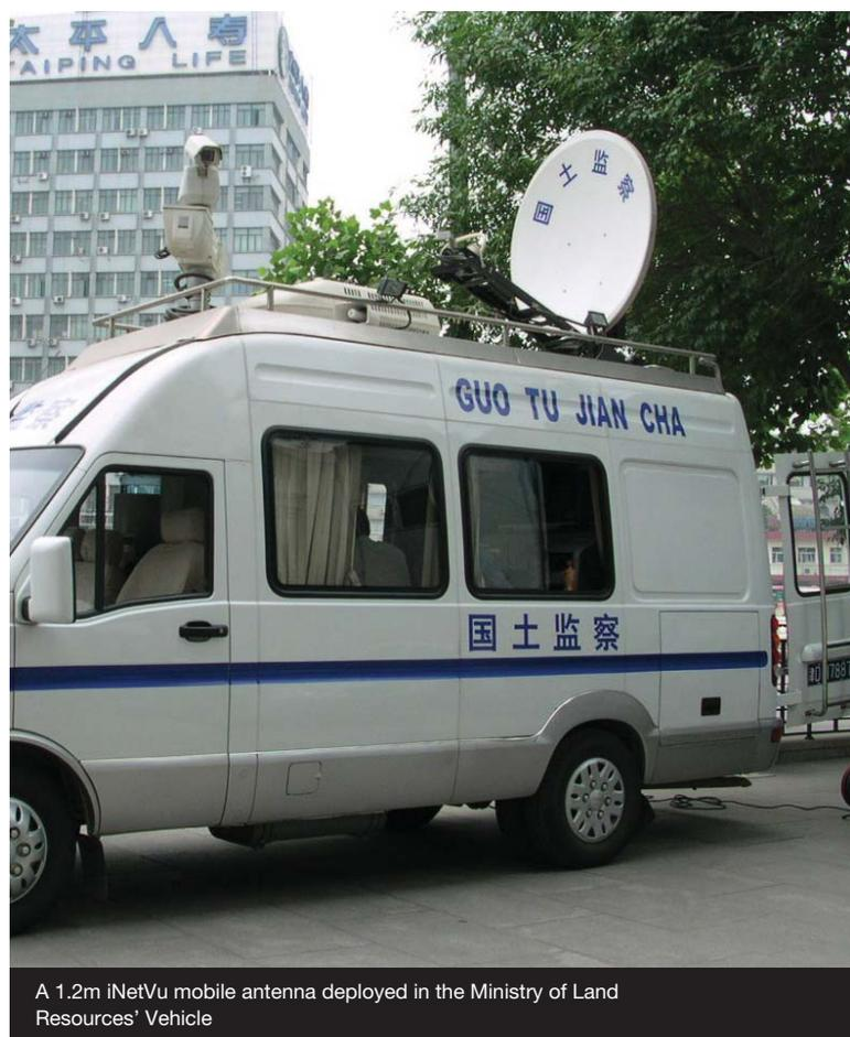
A 1.2m iNetVu mobile antenna deployed in the Ministry of Land Resources' Vehicle
