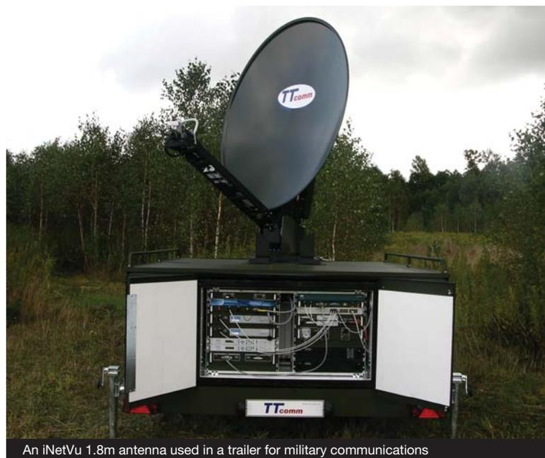
An iNetVu 1.8m antenna used in a trailer for military communications
